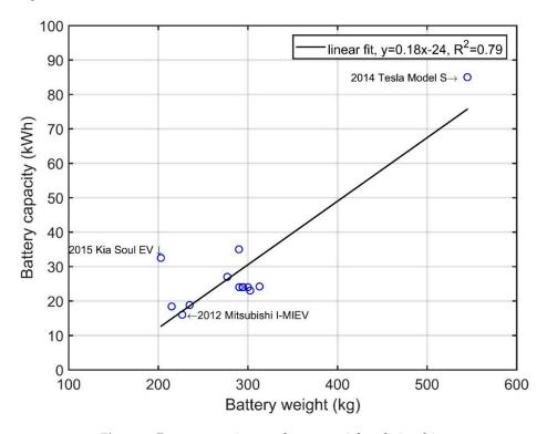
Figure 7. Battery capacity over battery weight relationship.
