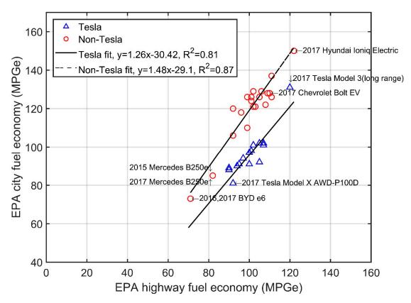
Figure 5. Correlation between EPA city mileage and EPA highway mileage for light duty BEVs.
