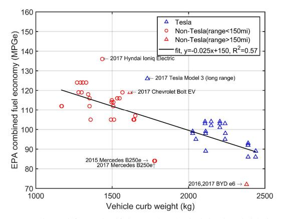
**Figure 4.** Scaling trend of EPA combined fuel economy (MPGe) with vehicle curb weight (kg). Blue represents Tesla vehicles, red represents non-Tesla vehicles, circle represents short-range BEV, and triangle represents long-range BEV.
