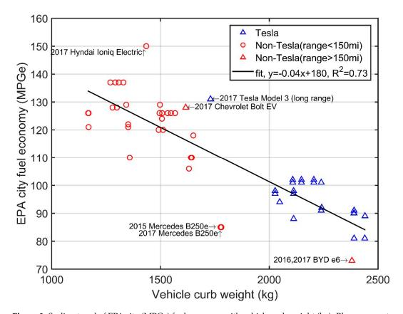
**Figure 2.** Scaling trend of EPA city (MPGe) fuel economy with vehicle curb weight (kg). Blue represents Tesla vehicles, red represents non-Tesla vehicles, circle represents short-range BEVs, and triangle represents long-range BEVs.
