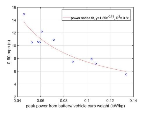
**Figure 6.** Acceleration for 0–60 mph (s) as a function of peak power from battery normalized by vehicle curb weight.
