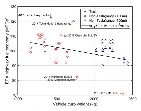
**Figure 3.** Scaling trend of EPA highway fuel economy (MPGe) with vehicle curb weight (kg). Blue represents Tesla vehicles, red represents non-Tesla vehicles, circle represents short-range BEV, and triangle represents long-range BEV.
