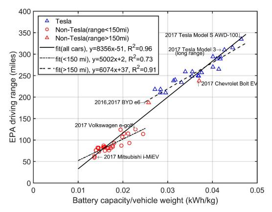
**Figure 1.** Scaling trend of EPA driving range (miles) per charge vs. battery capacity/vehicle curb weight (kWh/kg). Blue represents Tesla vehicles, red represents non-Tesla vehicles, circle represents short-range BEVs, and triangle represents long-range BEVs.
