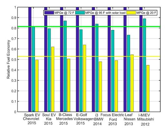
**Figure 8.** Effect of ambient conditions on BEV fuel economy. Yellow and green lines represent average values for MPGe at 95 F with solar load and 20 F respectively. The fuel economy was over the UDDS cycle.
